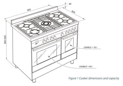
The cooker must be installed by a qualified technician and in compliance with local safety standards. This cookers has class "2/1" overheating protection so that it can be installed next to a cabinet.
